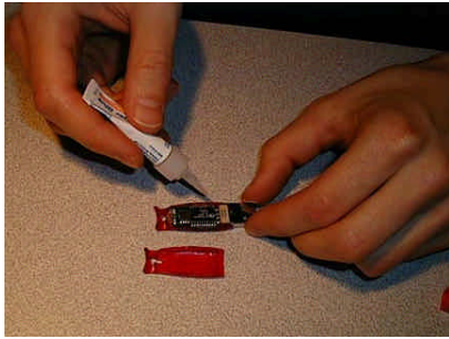
Figure 2e: After the electrical attack is complete, applying glue to both sides of plastic housing.
