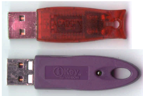
Figure 1: Aladdin Knowledge Systems' eToken R1, top, and Rainbow Technologies' iKey 1000 and 2000, bottom.
