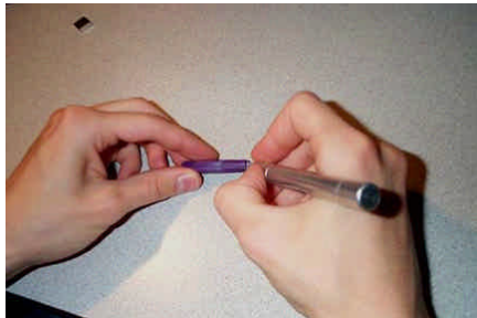
Figure 4c: Prying of the plastic housing.
