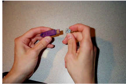
Figure 4b: Removal of the metal USB housing.
