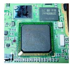
Figure 3: Glue around the edges of BGA packages on Sprint PCS phone
