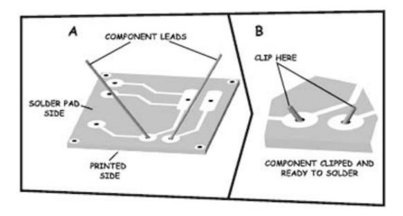
To prep your component for soldering, you need to feed it through the appropriate holes of your circuit board so that the component leads protrude from the solder pad side of the PCB (the component itself being on the printed side of the board). One way of getting the
