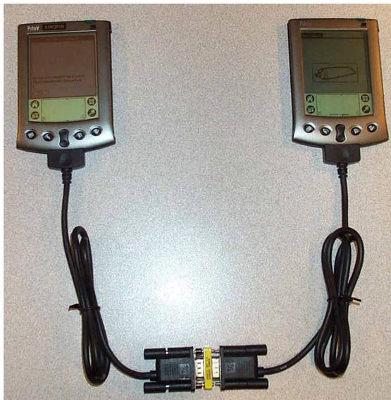
To connect the two Palm devices together, you will need to make a null modem cable to connect between the two using:
